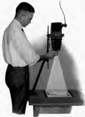
Fig. 4. Method of making an exposure with the Kodak Auto-Focus Enlarger. Turning down the exposure lever.
